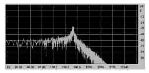
Spectrum of a noise signal proceed with a low-pass filter
