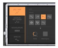
On the original synthesizer (equivalent to the "Classic" mode), oscillator3 can be set to the low frequency ("Lo" position in the range) to be used in LFO mode. This removed the possibility of using 3 simultaneous oscillators as well as a slow modulation on the filter cutoff frequency for example.
