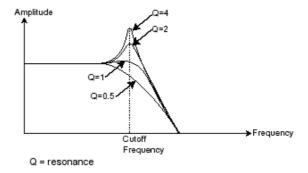
With a high resonance level, the filter will begin to produce a sound close to a sine waveform. At this stage, the use of a key follow is very important as you can create a melody by tuning the cut-off frequency of the filter with the frequency of the oscillators.
