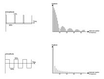
Time and spectral representations of the pulse and square waveforms
