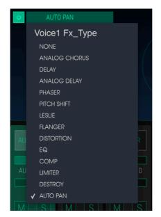
To enable or disable an effect, toggle the on/off button to the right of the effect name. This is sometimes referred to as a "bypass" switch. Audio will still pass through the disabled effect to the next effect or the mix output, but the effect itself will not affect the audio signal.
