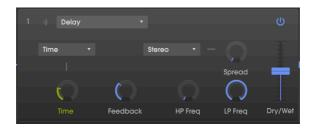
A delay can increase the spaciousness of a sound by providing distinct echoes within the stereo field. It can also be used as a rhythmic counterpoint to accentuate a groove. The Time options let you synchronize the delays with tempo and any other synchronized parameters of the CZ V, and even allow delays in triplet and dotted times.
