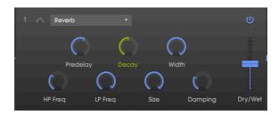
A Reverb effect creates a large number of echoes that gradually fade or "decay". It simulates how the input would sound in a room or a large space.
