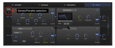
The same effect modules as in the first illustration, but in parallel mode. Line 1 is going through a Reverb into a Multimode Filter, and Line 2 is going through a Chorus into an Overdrive. Note the addition of the Line 1 and Line 2 volume controls on the right side.
