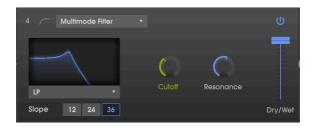
This analog filter model inserts one of 5 different kinds of filter into the FX chain. It can act in low pass, high pass, band pass, and two comb filter modes. Each pass filter is available in 12-, 24-, and 36 dB per octave slopes.
