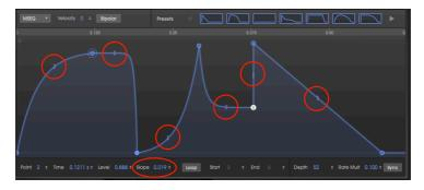
Double-click the numeric Slope field to reset a curve to a linear slope.
