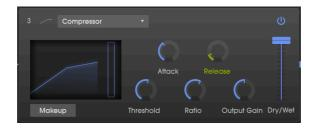
A compressor is an automatic level control. If a signal rises above a certain level (the threshold), the compressor lowers the signal output to compensate (at low Ratios) or won't let it rise at all (high Ratios, also called "limiting"). It is generally used to help maintain a consistent level of sound, though there are many other ways to use it.
