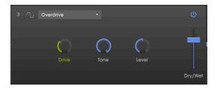
The Overdrive effect will add a certain "fuzziness" to the sound. The tone control will adjust the brightness of the output. This is modeled after a "solid-state" circuit being distorted.
