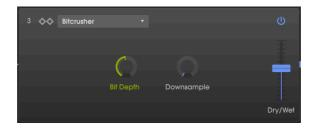
This bit-reducing effect offers several ways to deconstruct the sound. As the number of bits used to express the sound is reduced, details will gradually disappear.
