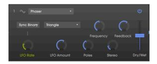
A phaser uses a steep multipole filter whose frequency can be modulated by an LFO, sweeping across the spectrum of the input, causing that familiar "whooshing" sound. It is similar to flanging, but is filter and phase-based instead of time-based.
