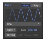
The CZ V has two independent low-frequency oscillators, in addition to the dedicated Vibrato LFO on the top panel. The parameters for LFO 1 and LFO 2 are identical, so the description of each parameter applies equally to both LFOs.
