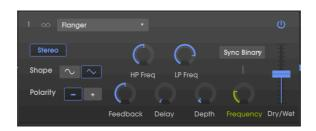
Flanging works by mixing two nearly-identical signals together, with one signal delayed by a small and gradually changing period. This produces a swept "comb filter" effect as the delayed signal adds and subtracts from the original due to phase cancellation at multiple frequencies simultaneously.
