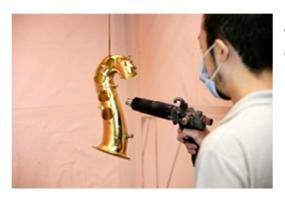
All parts are sprayed with a lacquer coat and then placed in an oven to heat-cure the lacquer.
