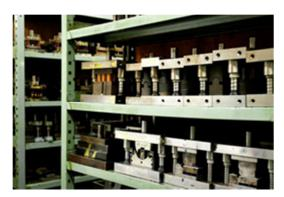
An assortment of press dies used to make various parts. Multiple dies are used in the production of each individual part. The factory uses over 2,000 dies in all.
