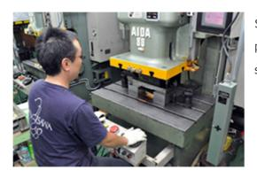
Sax key parts and certain body components are punched out on press machinery. Over 10 variations in thickness are used for such punched-out parts.
