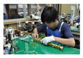
During assembly we apply a tape film to protect each instrument from scratches. Assembly proceeds with installation of the righthand keys followed by the left-hand keys and then the side keys.
