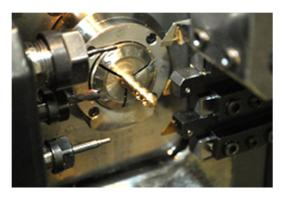
Sax posts of different sizes and shapes are cut to precision dimensions on CNC lathes.
