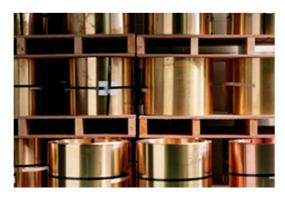
Rolls of metal sheet stock are sorted by brass, bronze, and silver alloy and utilized in different combinations depending on the saxophone model being made. Each roll is about 30 meters long.
