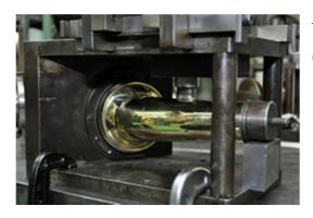
Tone hole locations are drilled into the shaped and polished body components after they are placed in a special die.
