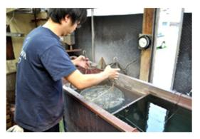
Prior to lacquering, everything is given an ultrasonic bath. This cleaning process completely removes all oils and buffing compound residues.
