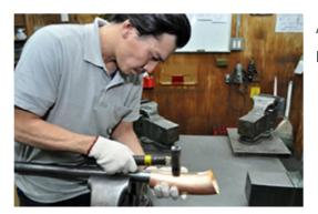
Any bumps or pits that remain after the welding stage are hammered and smoothed out to hide the joint seam.
