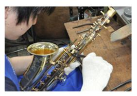
Preliminary key fitting is performed to enhance the precision fit of the key mechanism in the final assembly stage. The sax is also checked for silver-solder residues and flaws in the key mechanism.
