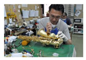
The assembly process is complete when the bell is attached to the instrument and the low-note bell keys controlled by the lefthand little finger are finally installed and regulated.
