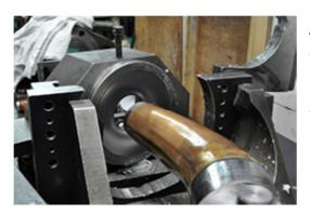
A metal mold is used to shape the body . An inserted tool forces the body through a slightly smaller-diameter hole in a metal plate. The hole in the plate is adjusted for changes in body taper.
