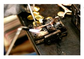
Over 120 different types of parts are created by silver-soldering key cups and other components to sax hinge rods and hinge tubing.
