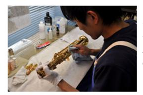
Following final inspection, the protective tape is removed and the sax is polished with a cleaning cloth to remove any fingerprints and smudges from the preceding work stages. Additionally, it will be checked over one last time for scratches or other blemishes.
