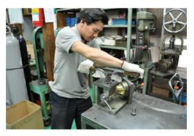
When the handle is turned, a round piece is pulled through to form and draw out the tone hole from the wall of the body tubing. Special care is the rule when fabricating tone holes because they have the most significant influence on the saxophone's scale.
