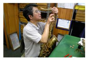
The instrument-making process concludes with a final, meticulous inspection of each fully assembled instrument. This inspection includes balancing the keys, tensioning the springs, and precision-fitting the neck.
