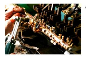
Post assemblies are soldered to the body with a 400 C torch.
