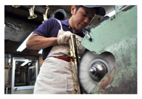
The body is polished in several steps with each pass utilizing a softer abrasive compound or buffing wheel.
