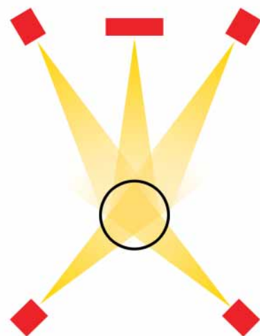
A narrow dispersion characteristic, such as that typically produced by other loudspeakers and especially sub-sat systems, will mean a very small listening area or 'sweetspot'
