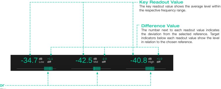
The indicator and the readout both turn green if the measured value meets the value of the reference.
