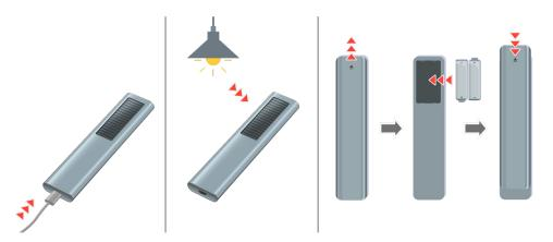
If you cannot see infrared signals, charge the remote control by using the USB port (C-type) on the bottom, or turn over the remote to expose the solar cell. If the remote control has batteries, replace them with new ones.
