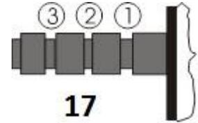
Slip the loop of the anti-skating weight's thread over the second groove of the stub to set the correct anti-skating force for the factory-fitted cartridge. Feed the thread through the loop of the wire support (15).
