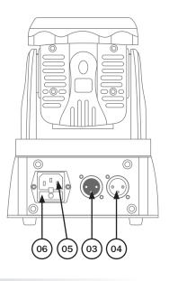
01 - LED display 02 - Function buttons 03 - DMX input socket 04 - DMX output socket 05 - IEC power input socket 06 - Fuse F5A 250V
