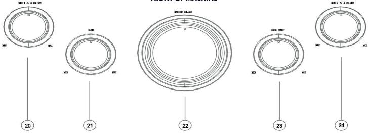
**20:** MIC 1 & 3 VOLUME knob controls the volume for microphones 1 and 3.
