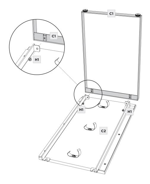
Connect (C1) Leg Frame to (C2) Top Panel inserts using 3 (H3) Screws. Fully tighten both (H1) Screws and (H3) Screws with (T1) Hex Wrench.
