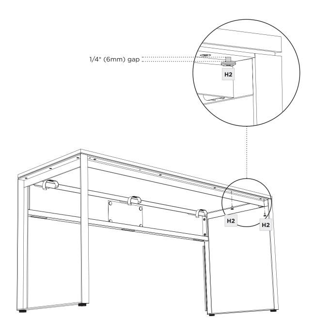
Slide the connection tabs onto the partially threaded screws. Tighten the **(H2) Screws** with the **(T1) Hex Wrench**.
