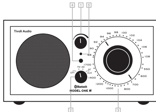
1. **VOLUME KNOB:** Rotate the volume knob to the right to increase the volume or to the left to decrease the volume. This knob also controls the volume of the headphone output.
