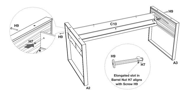
Step 5 - Secure Drawer Assembly A1 to Leg Assembly using Screw H8 and Hex Wrench T1. Insert Barrel Nut H7 into holes of Modesty Panel C10 with the elongated slot sitting vertically, and secure with Screw H10 through top of Drawer Assembly A1. Fully tighten all Screws that have been installed in previous steps using Hex Wrench.
