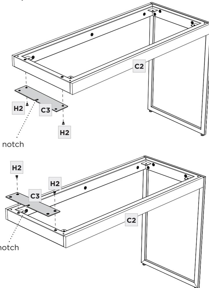
The return may be attached either to the **left** or **right** of the center drawer (**right side shown below**). Partially thread **1 (H3) Screw** into the **middle insert** leaving it extended out **1/4"** (6mm) to allow **(C3) Connector Plate** to slide into the space between the screw head and bottom of the desk.
