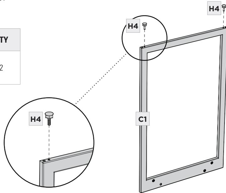
**ASSEMBLY****STEP 2. INSTALL TOP FRAME**
