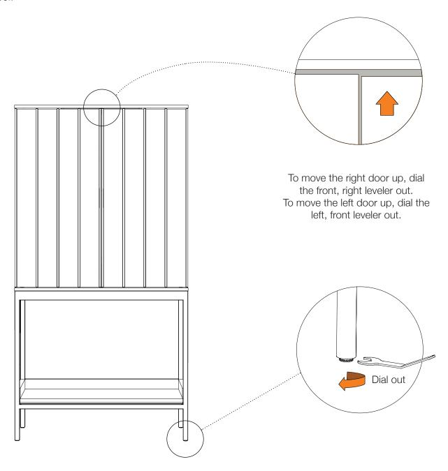
**Note:** To hold the doors in an open position, partially extend the two (2) front levelers. This action will tilt the cabinet back slightly, preventing the open doors from swinging towards their closed position.
