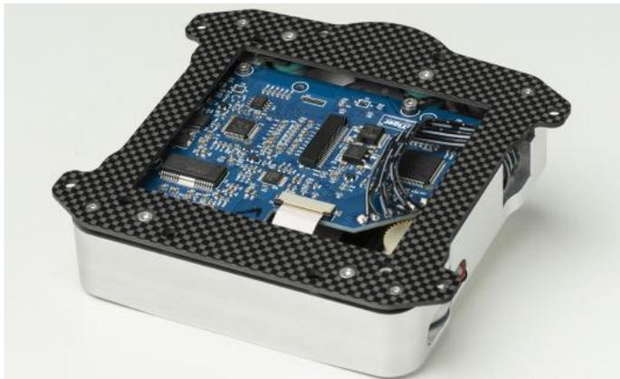
The suspension system consists out of a rigid carbon fiber plate, carbon fiber tubes, springs, silicon dampers and screws. The suspension, cover and turntable platter are made of 100% real carbon fibre.
