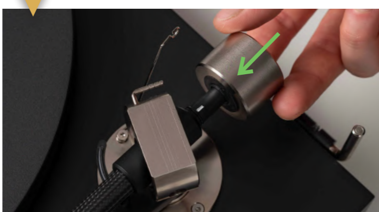
17 Balance the tonearm by turning the counterweight forwards and backwards on the rod.
