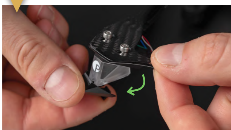
18 When the gauge stays level, your tracking force is set correct.
