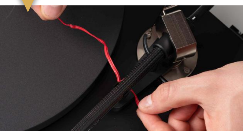
16 Place the stylus on the gauge. The stylus should read 20.
