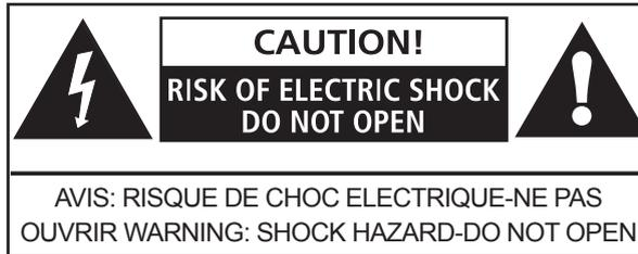
This lightning flash with arrowhead symbol within an equilateral triangle is intended to alert the user to the presence of non-insulated “dangerous voltage” within the product’s enclosure that may be of sufficient magnitude to constitute a risk of electric shock.
