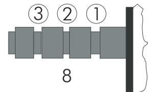
Hang the loop of the thread of the anti-skating weight in the groove of the anti-skating stub (15) corresponding to the downforce applied to your cartridge and hang the thread in the groove of the wire support (17).
