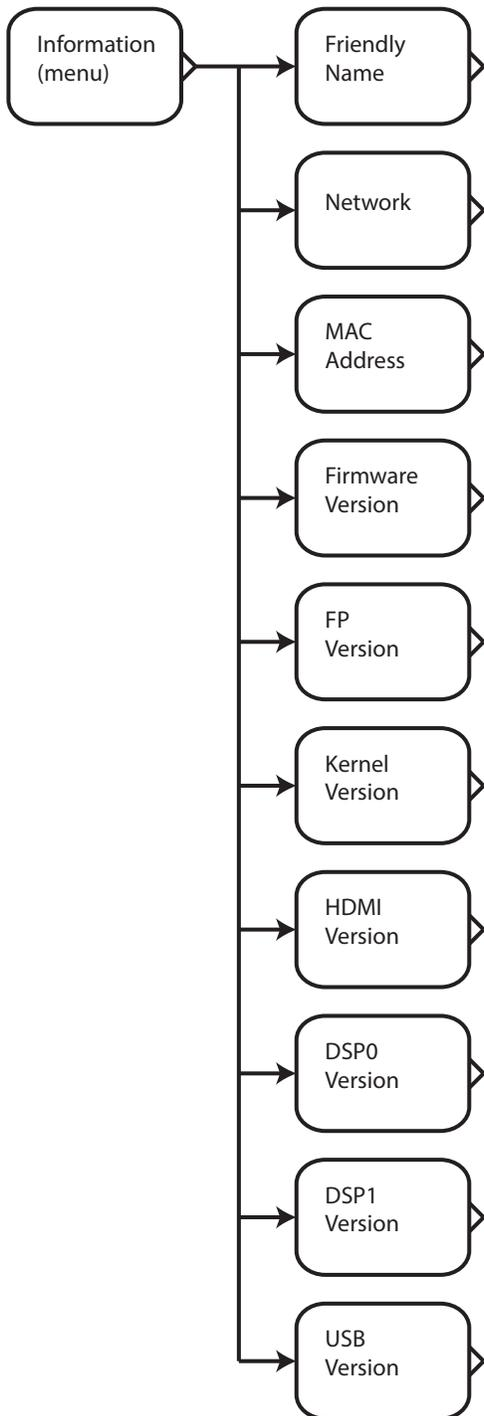
The **Information Menu** gives you access to information about the current Network configuration of the XMC-2, shows the versions of the currently installed firmware modules, and allows you to see the XMC-2's Friendly Name.
