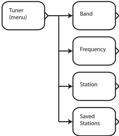
The **Tuner Menu** is used to select a station on the XMC-2's built-in high quality AM/FM tuner, and to create, rename, and delete station presets.
