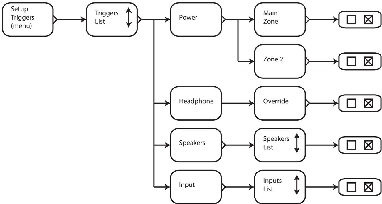
The **Setup Triggers Menu** allows you to configure how the triggers on the XMC-2 operate.
