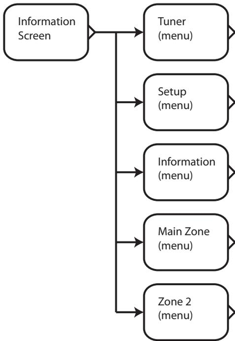
The XMC-2 **Menu System** is displayed by pressing the Menu button, and is displayed on the XMC-2 front panel display and the on-screen display. The Menu System is divided into five major functional categories.
