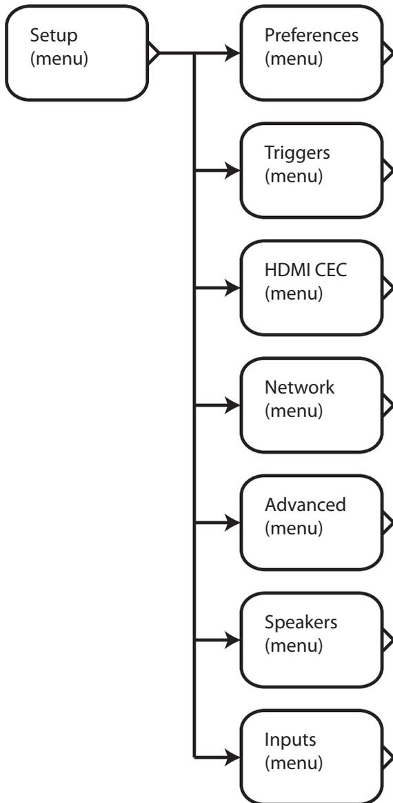
The **Setup Menu** allows you to view and change the main configuration settings for the XMC-2.
