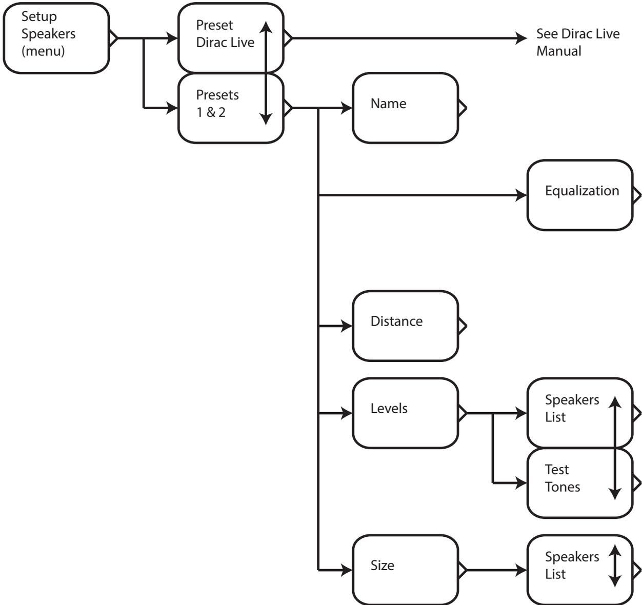
The **Setup Speakers Menu** is where you access the powerful speaker and room correction features of the XMC-2, including Dirac Live automatic room correction, and the XMC-2's incredibly flexible manual calibration system, which includes two fully independent banks of parametric equalizers, along with pink noise and test tone generators.
