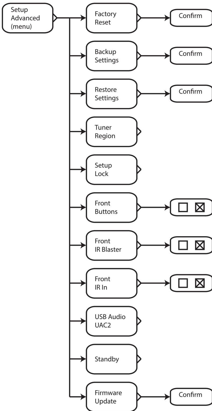
The **Setup Advanced Menu** allows you to configure various system operating preferences, including selecting a Standby Mode, and enabling various controls and remote control inputs and outputs. Firmware updates, and resetting your XMC-2 to factory defaults, are also initiated from this menu.
