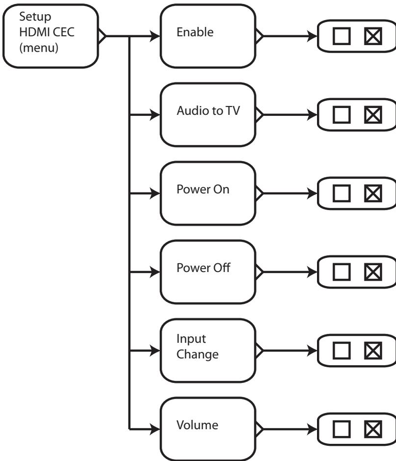
The **Setup HDMI CEC Menu** allows you to configure what types of CEC commands the XMC-2 sends and responds to.
