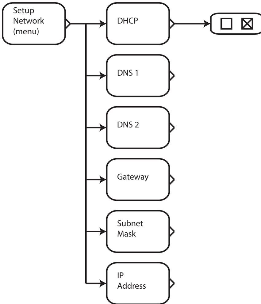
The **Setup Network Menu** allows you to configure various network parameters for the XMC-2.
