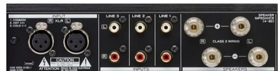
The AX-505 is also equipped with a set of wide-pitch, diagonally offset (for easy wiring) screw-type speaker terminals, capable of accommodating high quality AWG8 gauge cables and banana plugs.
