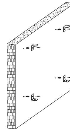
Use your measurements from step 8 to correctly locate the wall section of the bracket and mark locations for fixing / drilling.
