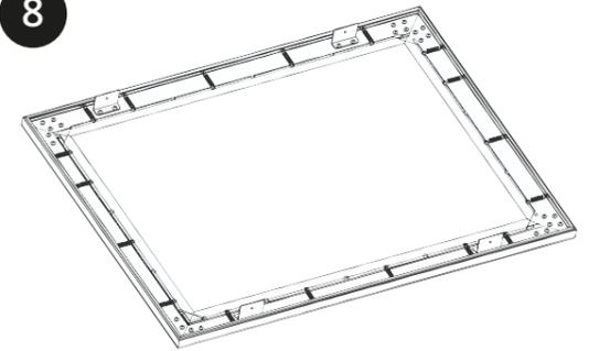
Measure the horizontal and vertical positions of the bracket locations on the screen.
