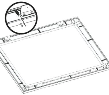
Install the springs on the four corners and middle position of each side first.
