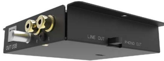
Take care to connect the left and right channels correctly. The right channel is usually marked red, the left channel black or white. Check the manual supplied with your amplifier for relevant information. The earthing wire of the tonearm lead should be connected to the earth terminal on your amplifier (if provided).
