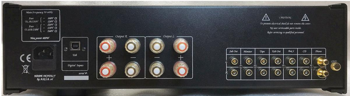
The Unico Due offers four inputs: three analogue inputs and one USB digital input. The input selection uses sealed miniature relay switches to preserve the delicate low-level signals, whereas the volume regulation is based on an integrated high-precision, high-performance resistor array followed by a set of digitally controllable analogue switches, used in reference products and capable of 120 dB of attenuation with 0.5dB steps.
