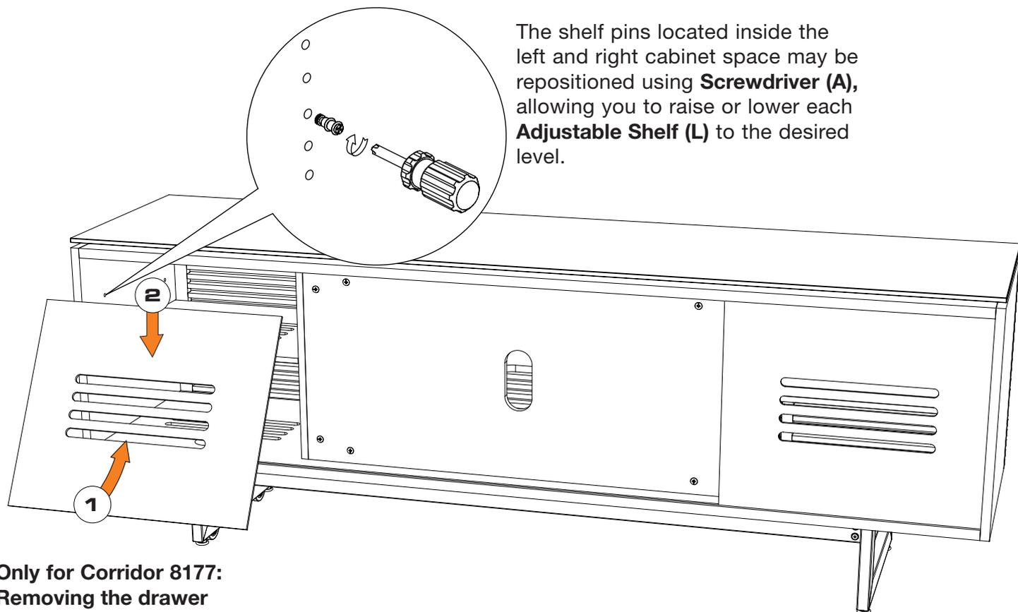
The shelf pins located inside the left and right cabinet space may be repositioned using **Screwdriver (A)**, allowing you to raise or lower each **Adjustable Shelf (L)** to the desired level.
