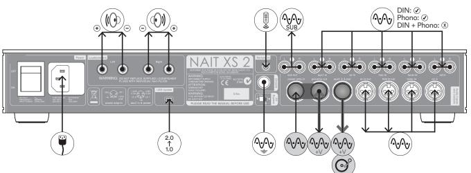
Note: The link plug should be removed only if a power supply upgrade is to be used, an alternative preamplifier is to use the NAIT XS 2 power amplifier section, or an alternative power amplifier is to use the NAIT XS 2 preamplifier section. It should remain fitted in all other circumstances.
