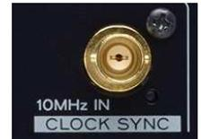
In addition, an external 10MHz clock input is also provided, to synchronise with an even higher-precision master clock generator, such as the TEAC CG-10M, for yet further upgraded audio playback with excellent sound quality.
