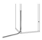
③ Run the speaker cable through the tube positioned at the rear of the cabinet to the terminal at the front baffle.
