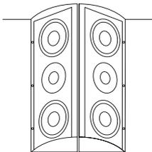
Likewise, three cabinets can be mounted together to cover 270 degree around a corner. Simply couple three cabinets together using the 9x3mm bolts and mount the speakers to the wall with the integrated mounting points.
