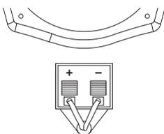
Connect the red (+) speaker cable to the red cable terminal and the black (-) speaker cable to the black speaker terminal.
