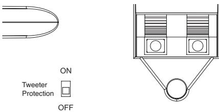
To enable, move the PTC switch to ON and to disengage, move the switch to OFF.
