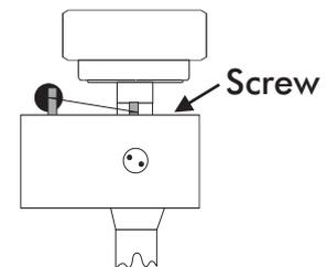
With the aid of a good magnifying glass adjust the needle until it is vertical in the groove (i.e. perpendicular to the record's surface). Ideally this should correspond to the top surface of the cartridge body being parallel to the record surface.
