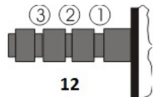
Hang the loop of the thread of the anti-skating weight into the groove of the anti-skating stub (12) corresponding to the downforce applied to your cartridge and hang the thread into the groove of the wire support (14).
