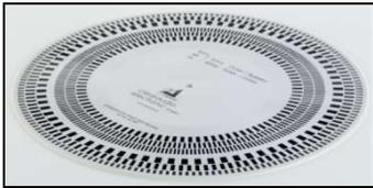
If you choose the side without the speed light source, you can use the regular light source for the installation, either 50 Hz (outer scales) or 60 Hz. The scales are graduated in three different reading options: 33,3 Hz, 45 Hz and 78 Hz (starting from the outer diameter).
