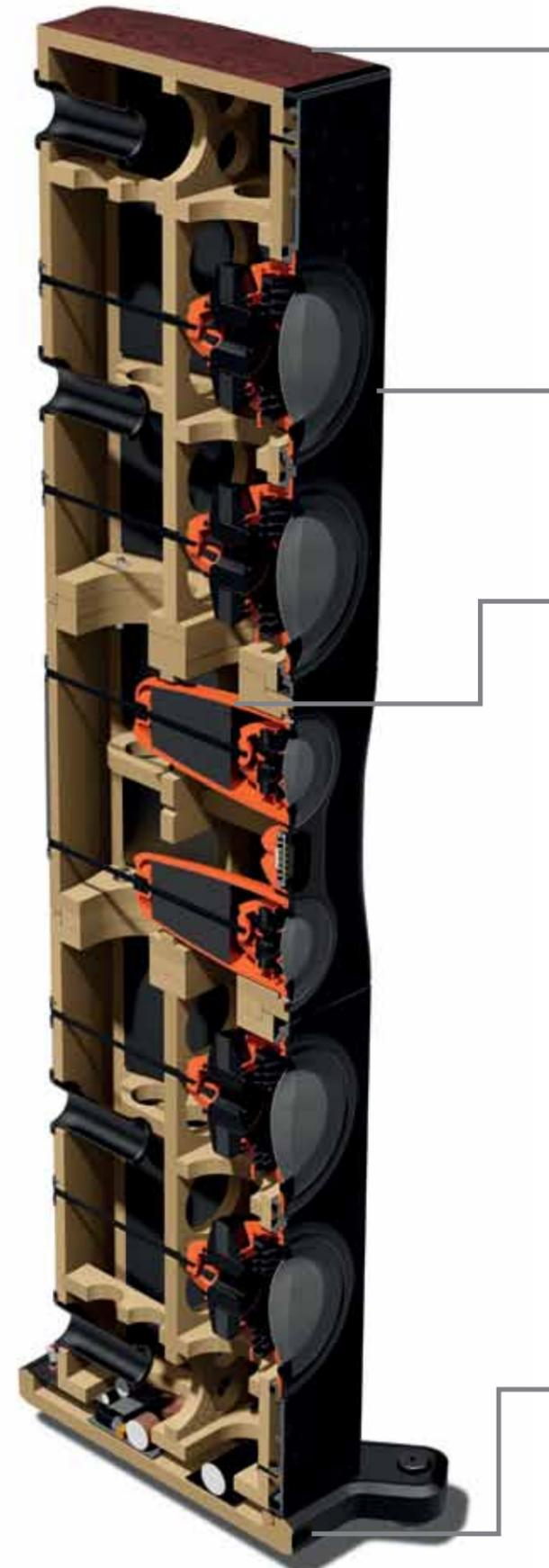
**CURVED AND BRACED CABINET CONSTRUCTION:** Curved surfaces are inherently stronger than flat surfaces, and since the internal sides are non-regular, standing wave formation is suppressed. New internal bracing structures have been developed to ensure the ultimate in structural integrity, and bitumastic damping material applied to all internal cabinet walls to ensure that all cabinet vibration is absorbed. Result: a supremely rigid, acoustically inert enclosure for natural, true-to-life fidelity.
