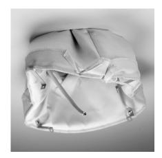
Grasp the firehood by its sides & squeeze it inwards to reduce its bulk. Then push it through the aperture with its top uppermost, ensuring that a grip on the fitting clips is mainained through the process.
