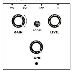
**TONE -** At higher settings this control adds openness, note articulation and picking detail. In this setting the top-end in your amplifier is sweetened while remaining smooth, the mids become focused, and the bottom end appears more robust and tight. At lower settings the Tone control can be used to fatten up an amp or tame harsh top-end.
