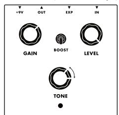
**GAIN -** Sets the input gain from off to maximum. With the Boost switch in the down position (VCA mode), this knob should be set to maximum. In this setting you will notice tighter bottom, focused midrange, and a more open top end. With Boost in the up position (clipped OTA mode), the sound is creamy and lightly compressed with a slightly more forward midrange.
