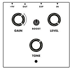
**LEVEL -** Level allows you to trim the output of the Boost while maintaining input gain coloration and compression. This control does not go completely off.
