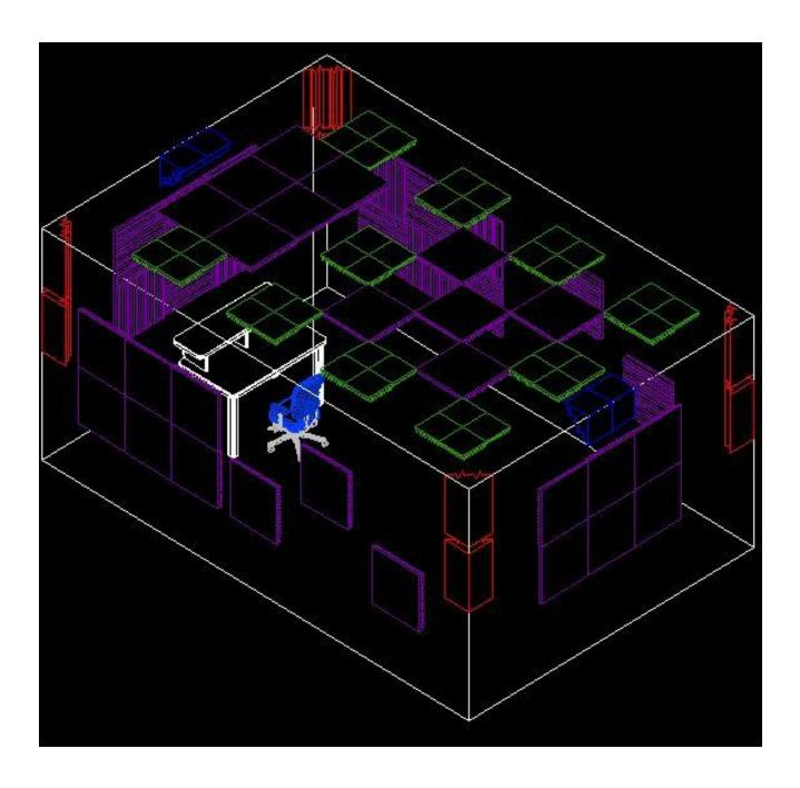
The pattern shown in this rendering is only one example of the way that the panels and bass traps of your Mercury-6 kit can be oriented in the room. If you desire a different aesthetic pattern, you can rotate the panels however you like as long as the guidelines listed above are followed as this will not detract from the performance of the acoustic treatment. Universal Acoustics foam materials will not only dramatically improve your acoustics but can also make your workspace look great.
