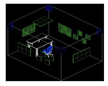
The pattern shown in this rendering is only one example of the way that the panels and bass traps of your Mercury-2 kit can be oriented in the room. If you desire a different aesthetic pattern, you can rotate the panels however you like as long as the guidelines listed above are followed as this will not detract from the performance of the acoustic treatment. Universal Acoustics foam materials will not only dramatically improve your acoustics but can also make your workspace look great.
