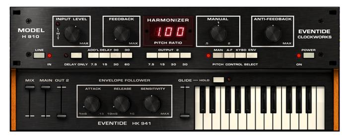
The H910 user interface consists of two parts. The top half of the interface is the front panel of the original H910 2U rack mount unit. All controls function in the same way as the original. The bottom half of the interface enables features originally available through external connections or options.
