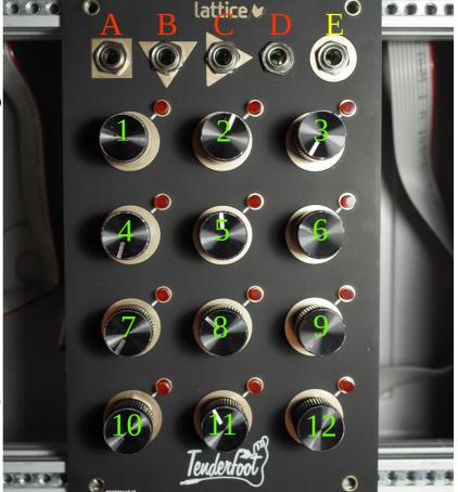
Output is the output of the module, where the control voltage generated by the sequencer is sent to. This is where you attach the module you wish to modulate (for example, the 1V/oct input of a VCO can be patched directly to the output of the Lattice here).
