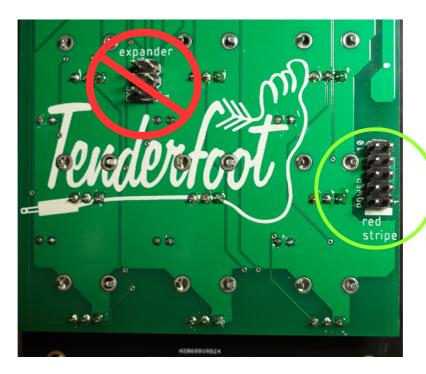
The POWER header is labelled at one end with a bold stripe, and the words "red stripe". Align the red stripe on the ribbon cable with the "red stripe" label on the PCB.
