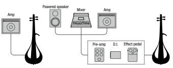
\* The input impedance of the first device (preamp, direct box, etc.) the instrument connects to has a major influence on the sound quality produced by the speakers. In order to obtain the maximum performance from the instrument, we recommend connecting to a device with an input impedance of more than 1MΩ.
