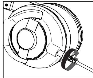
1. Insert 1/8" connector into socket (from cable or headphone volume control)
