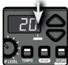
When JamMan Solo XTs are initially connected via the JAMSYNC jacks, 54n will appear in the slave's display, indicating JamSync connection is established. The 54n indicator will also be displayed when initially powering up devices which are slaved to a master. Properly connected slaves will also be indicated by a decimal segment which will light in the display, as shown to the left. If you have a slave connected and do not see these indicators, check your JamSync cable.
