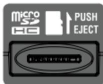
1. Fully insert the memory card into the card slot, contacts face down, and press until it seats solidly.
