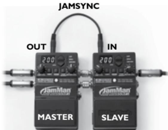
To use JamSync, connect the master JamMan Solo XT's **JAMSYNC OUT** jack to the **JAMSYNC IN** jack of the first slave device. Daisy chain any remaining JamSync slaves in the same manner.
