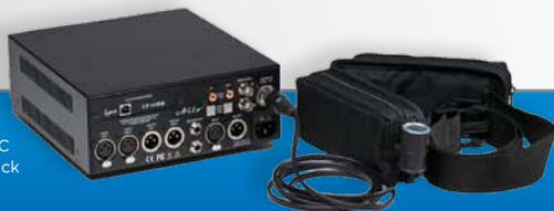
Hilo can be powered by AC or optional DC battery pack
