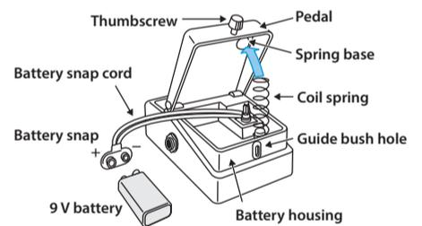
1. Hold down the pedal and loosen the thumbscrew, then open the pedal upward.
