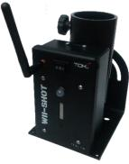
2. Set the power switch to wireless mode [II]. Be sure there is enough battery charge. The status LED on the WII-Shot will be blinking in blue, this means it will accept a mating call from the controller. If you do not mate the WII-Shot within 60 seconds, the WII-Shot will shut down to save battery power.
