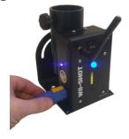
4. In order to keep the battery healthy it is important to charge the device as soon as there is no charge left. When not in use for long periods of time, please check the battery level every few months to compensate for any natural self-discharge. Leaving the battery without charge for long periods of time can cause irreversible damage.
