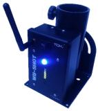
3. Switch on the controller. Some of the four red buttons will illuminate, this indicates the controller's remaining battery charge. (1=25%, 2=50%, 3=75%, 4=100%)
