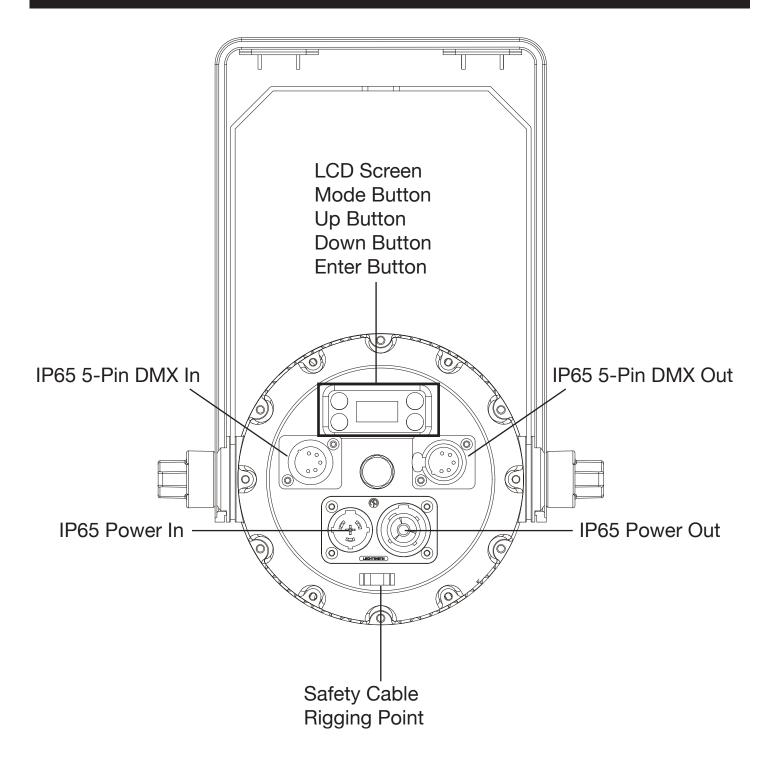
Always ensure that the unit is firmly fixed to avoid vibration and slipping while operating. Always ensure that the structure to which you are attaching the unit is secure and is able to support a weight of 10 times the unit's weight. **ALWAYS** use safety cables that can hold 12 times the weight of the unit when installing the fixture. This equipment must be installed by a professional, and it must be installed in a place where it is out of the reach of people's grasp.
