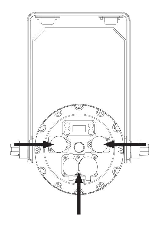
**DMX-512:** DMX is short for Digital Multiplex. This is a universal protocol used as a form of communication between intelligent fixtures and controllers. A DMX controller sends DMX data instructions from the controller to the fixture. DMX data is sent as serial data that travels from fixture to fixture via the DATA "IN" and DATA "OUT" XLR terminals located on all DMX fixtures (most controllers only have a DATA "OUT" terminal).
