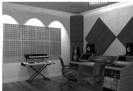
Eight Radiator diffusers are bolted together and hung on the wall to create ambience in the studio.
