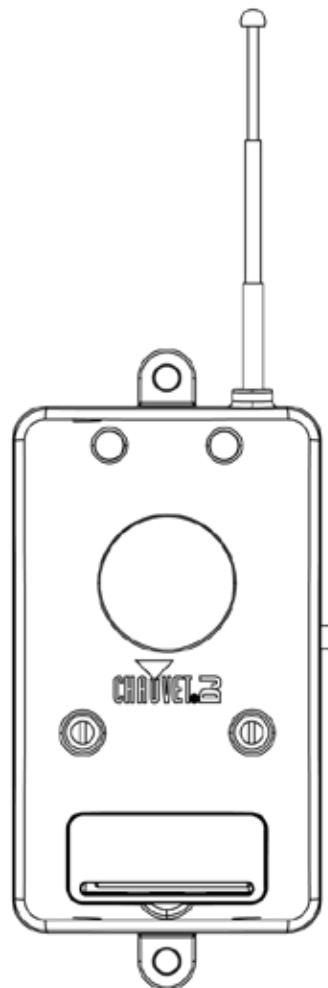
The WMS (Wireless Motion Sensor) allows you to trigger compatible foggers with motion activation. This consists of the transmitter with built-in delay time and sensitivity knobs for control of up to 4 fog machines independently. More may be run if addressed simultaneously. See the instructions below to set up your fogger to operate with the WMS.
