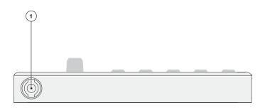
1. BATTERY DC In, Input for accessory battery power supply.
