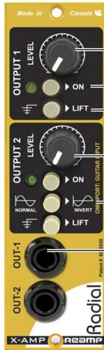
**FULL ENCLOSURE** - 100% steel casing reduces magnetic interference from other nearby modules that may cause pollution.
