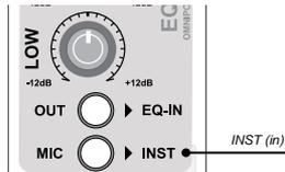
The MIC/INST selects between the XLR mic input and the Omniport instrument input.
