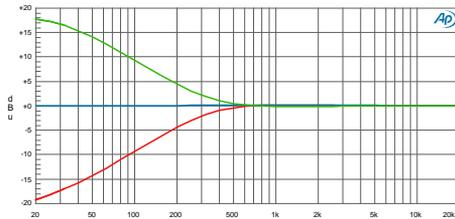
The high frequency control makes it simple to add extra sparkle to a 12-string acoustic guitar or reduce the shrillness of a violin. The low frequency control can boost the bottom end of a male voice or be used to fatten a bass guitar. Cutting some mid-range can pull a track back into the mix, while boosting mid-range brings it forward.
