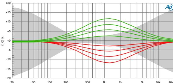
The mid-range is superimposed over the high and low filters to show the frequency overlap between bands.
