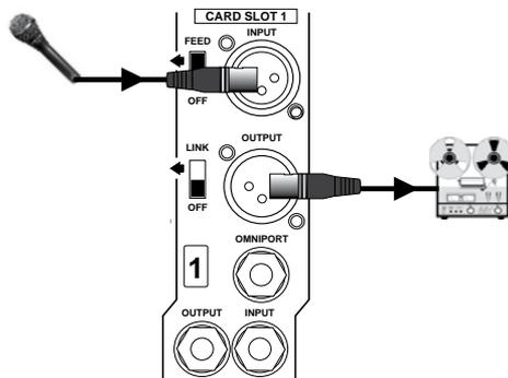
*Rear panel mic input and line output.
